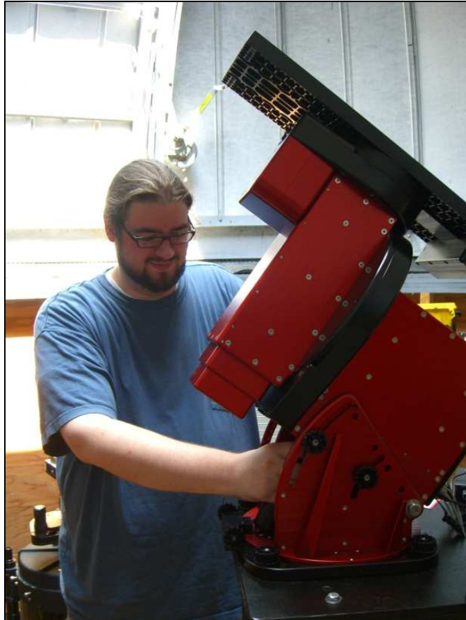
FIG. 14. The author adjusting the altitude on the Paramount ME after installing it in the DSO-14 dome. (D. Caton)
