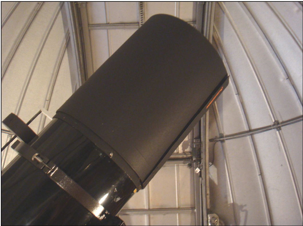
FIG. 21. Celestron C-14 Lens Shade/Dew Shield prevents dew and dust from accumulating on the corrector plate and improves image contrast by keeping out stray light. (Author)
