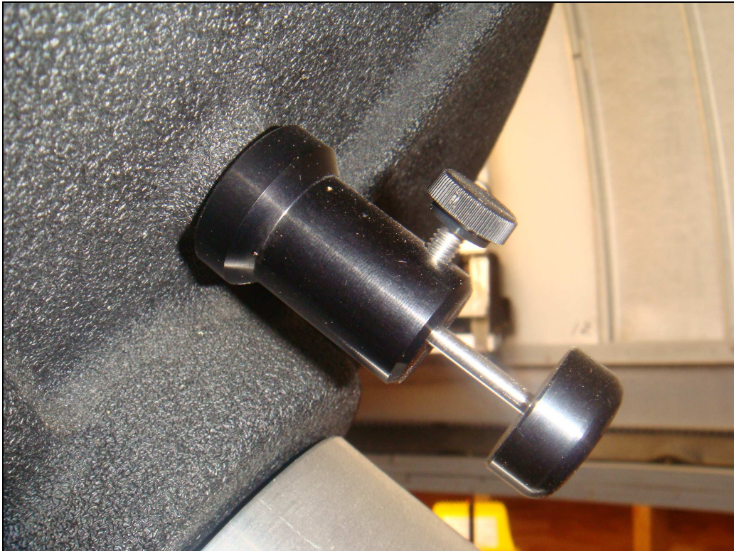
FIG. 23. One of the two C-14 Flopstoppers holding the primary mirror in place. (Author)
