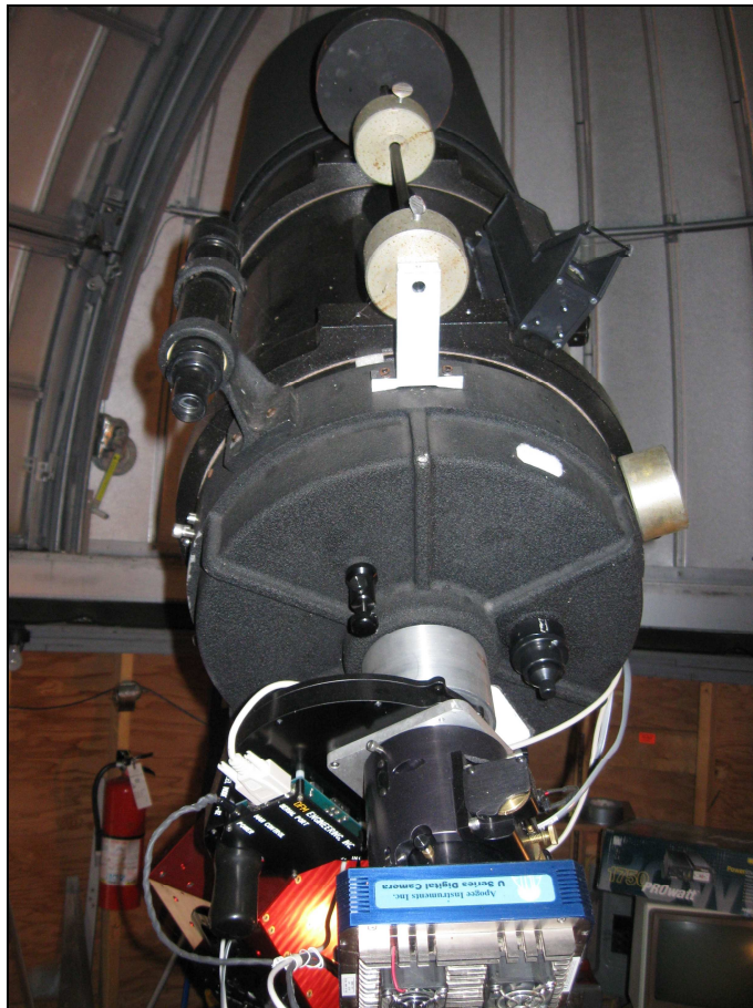
FIG. 28. Image showing the counterweight (steel weight on right side of image) used to negate the weight from the filter wheel (bottom left) being off axis. (Author)
