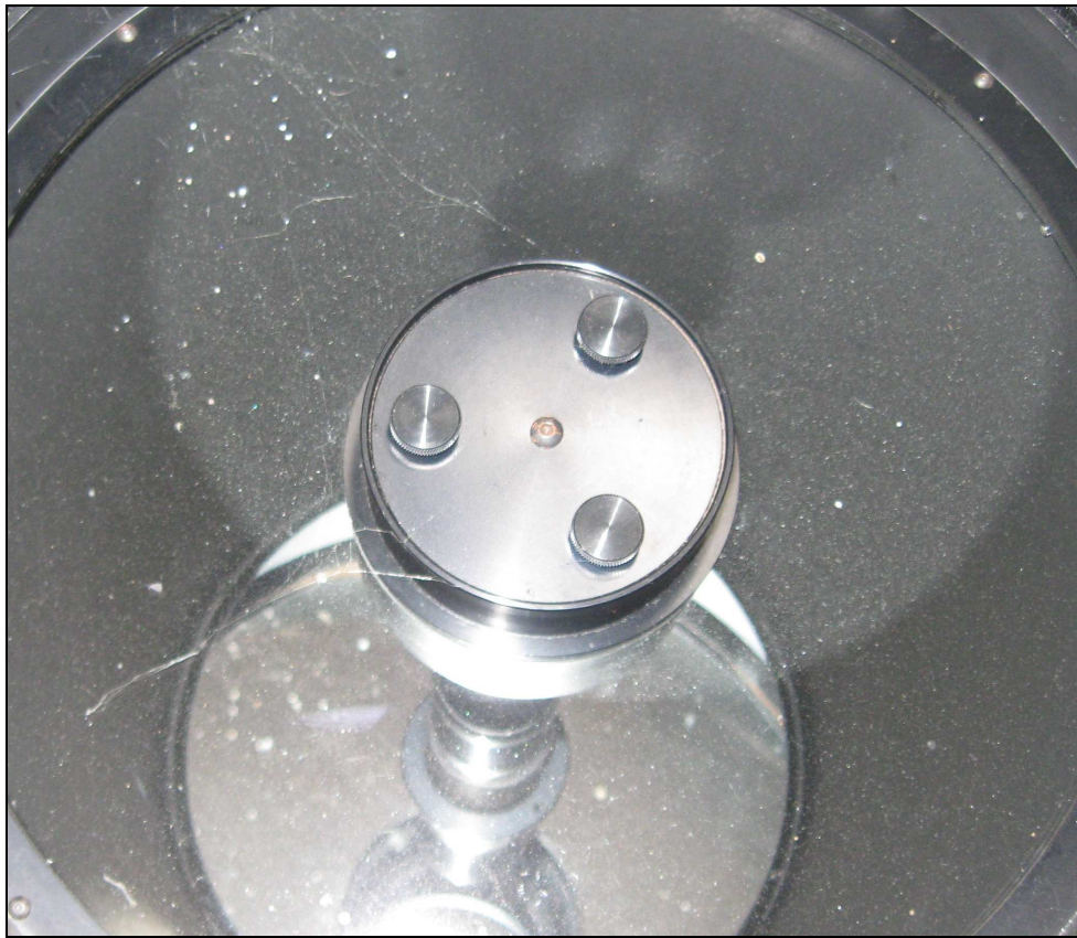
FIG. 22. The collimation thumbscrews on the secondary mirror make collimation a much easier task. (Author)
