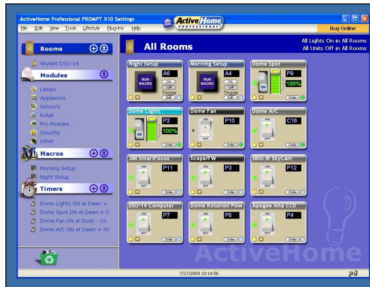
FIG. 70. ActiveHome Professional is the software that we use to control the X10 modules. With it we have set timers to automatically turn off the lights two hours before sunset (to allow for darks to be taken in a darkened dome) and to turn on at sunrise. (Author)
